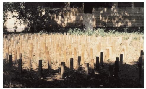
Figure 1. Field test. Samples treated with CCA type product exposed in the test site 290
