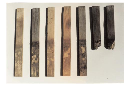
Figure 4. Spruce samples after 24 month of exposure in ground contact
