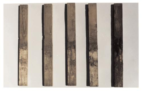
Figure 2. Pine sapwood samples after 24 month of exposure in ground contact
