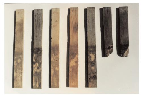
Figure 3. Beech samples after 24 month of exposure in ground contact
