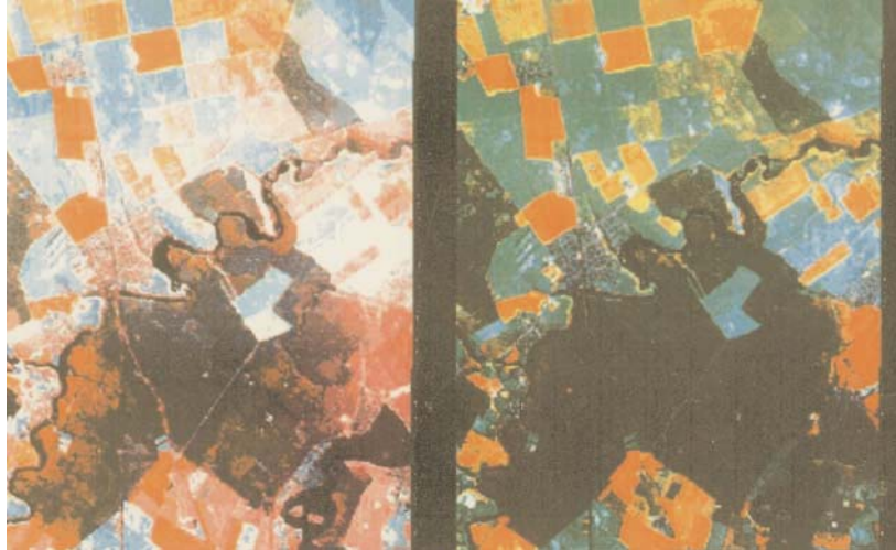
Figure 2. Landsat TM 4/5/3 for Cernica area without atmospheric correction (left side image) ; with atmospheric correction (right side image).
